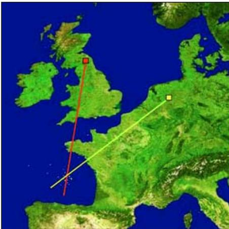
Figure 2 - Lightning Location by Triangulation
