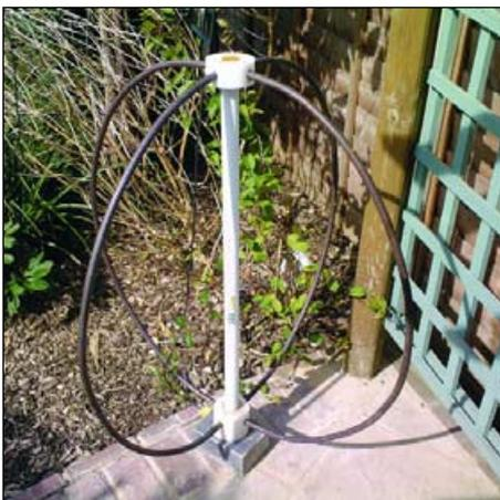
Figure 5 - The Copper-Pipe Loop Antenna
